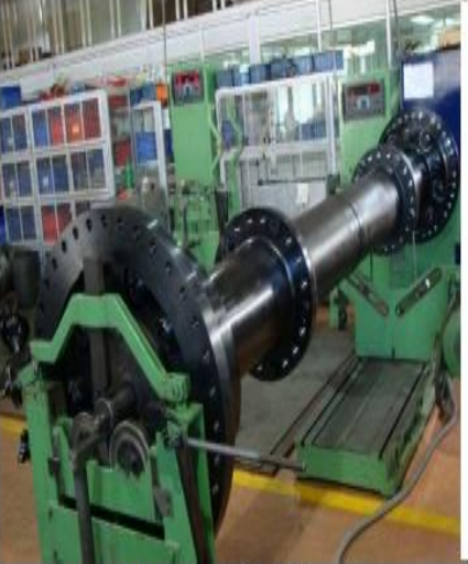
Coupling with large DBSE (6 Mtr)
